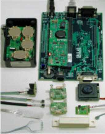
"Tini" micro-controller and sensors embedded in cabinetry
