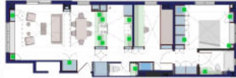
Environmental Sensors: CO, Co2, Temp., Humid., etc.
